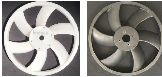
Fig. 4. The fan produced by centrifugal casting and reference fan
