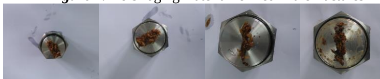
Figure 2. Bridging material formed in the fractures
