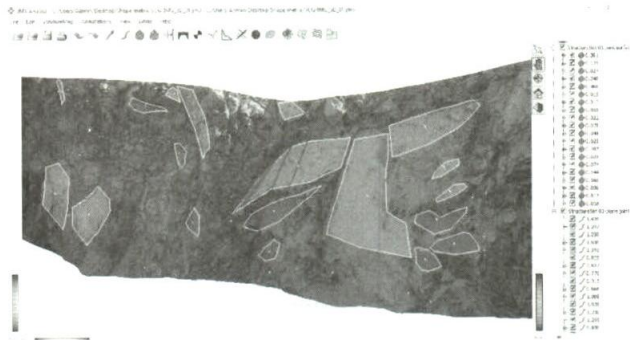
Figure 5. A 3D photograph formed shows discontinuities at zone E in the software.
