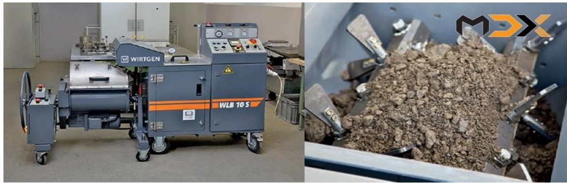
Fig. 3. Laboratory mixer for recycled aggregate blend used in foamed bitumen content design
