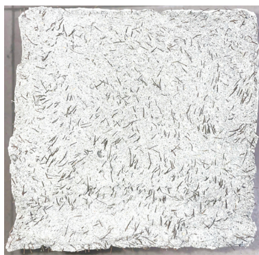
(a) Cross-section at crack path (F2C0)
