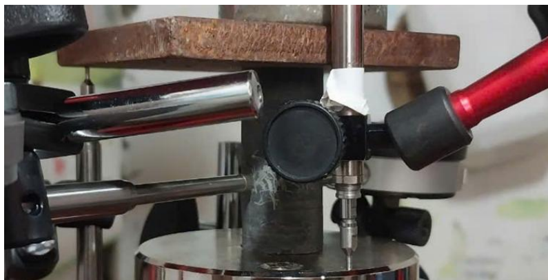
Fig. 3. Sample machining and loading, installation of a displacement measuring gauge, compression force.
