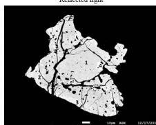
Fig. 4 BSE image of uraninite with points of absolute age calculation.
