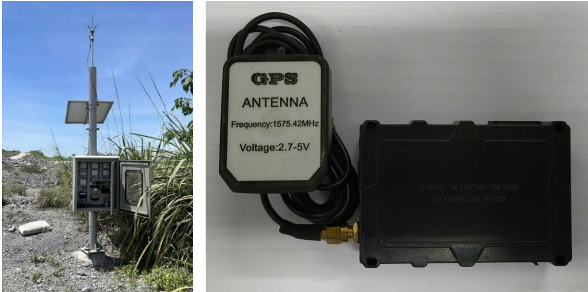
Figure 1. Monitoring Station and GNSS Device
