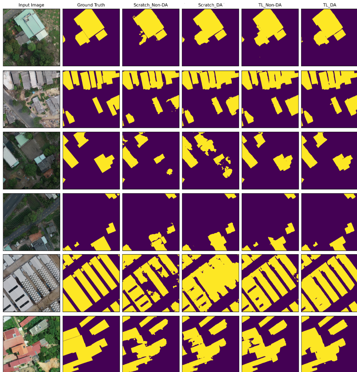
Fig. 7. Comparison of predicted masks from the four training methods scenarios, including training from scratch and transfer learning without and with data augmentation
