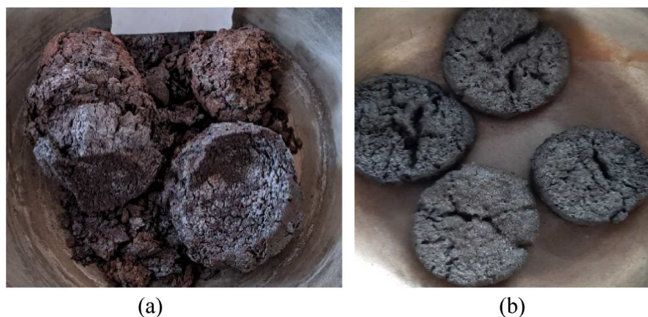
Figure 7. Sample image after reduction at 1100°C. a. With no additives; b. With the use of \text{Na}_2\text{SO}_4 additive.
