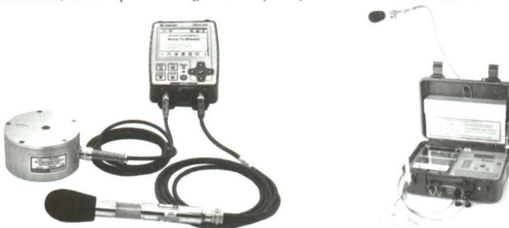
Figure 3. Equipment Used for Monitoring Blast-Induced Ground Vibrations
