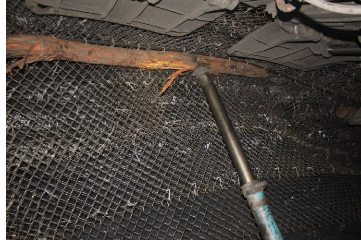
Fig. 1 Longwall face in Vang Danh coal mine, Vietnam: stability (left, no mesh) and instability (right, with mesh)
