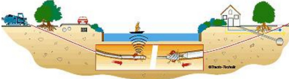
Figure 1: Horizontal Directional Drilling scheme (Tracto Technik 2010)
