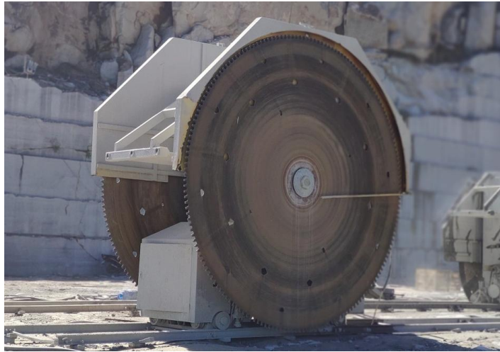
Fig. 4. Combination between disc sawing and diamond wire machines in a dimension stone quarry
