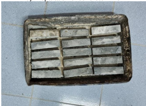
c) Specimens with dimensions of 40 x 40 x 160 mm (ECC1)
