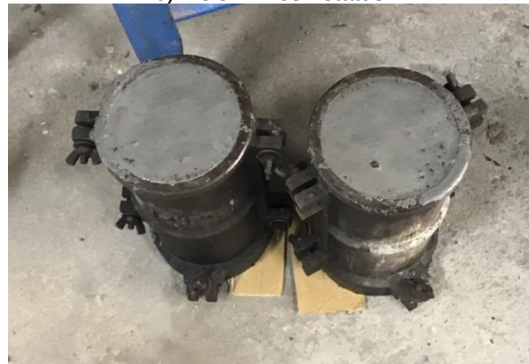
d) Standard specimens with dimensions of 150 x 300 mm (ECC2)
