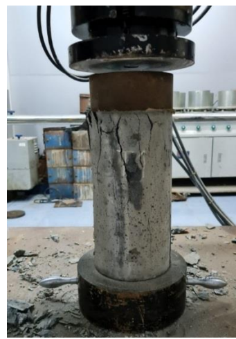
b) Failure mode of ECC specimens
