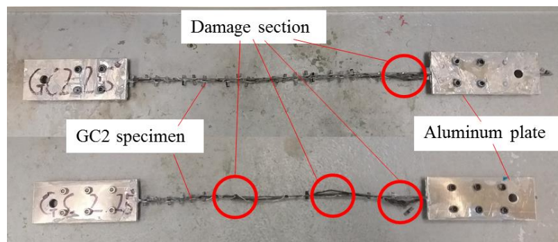
b) Failure mode of GC2 carbon textile under tensile loading at room temperature
