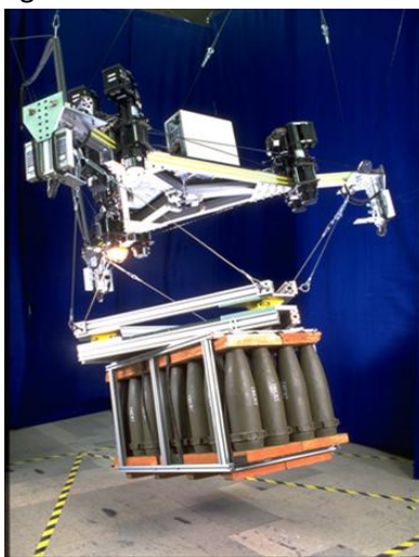
Figure 1 – Crane robot transports goods
